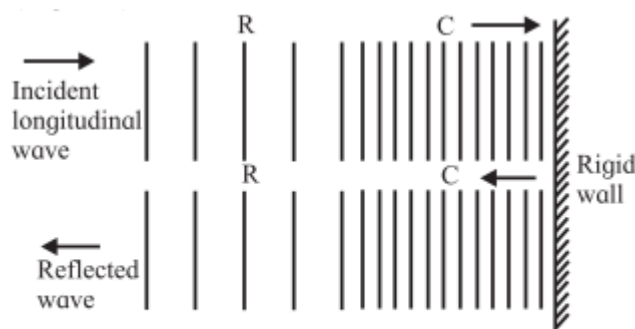
Fig. 6.4: Reflection of a longitudinal wave from a denser medium.
